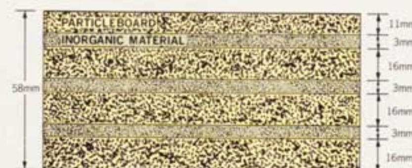
Cross Section of Multi-Layered Cabinet
