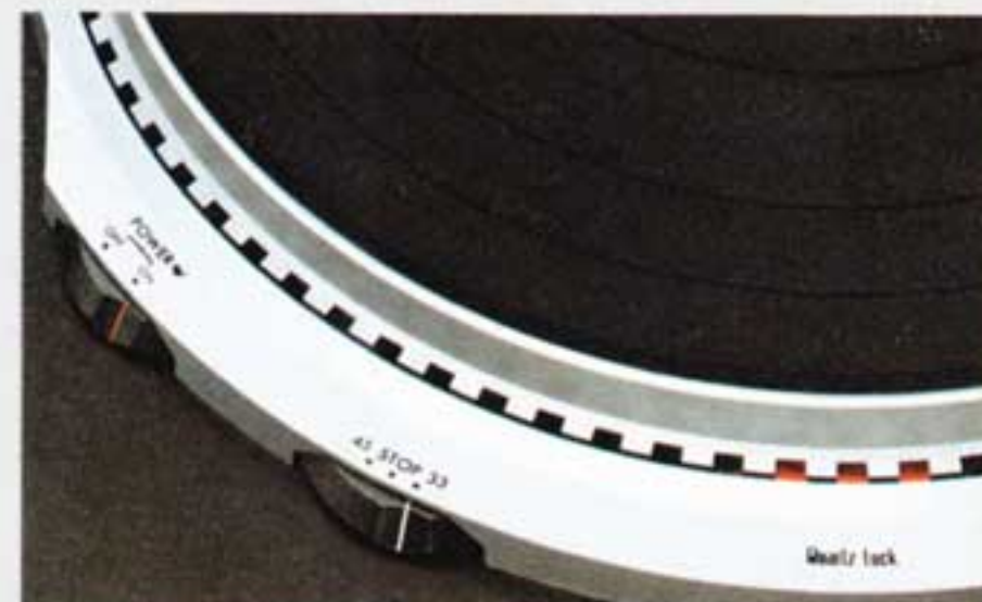
Power On/Off & Speed Switches
