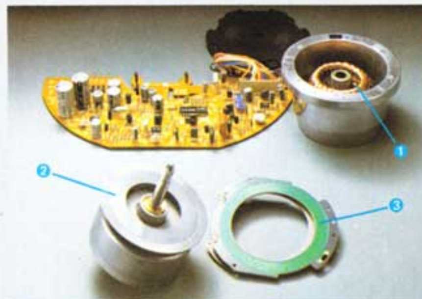
JVC Super Servo Frequency Generator 1 24-Slot Stator Coil 2 Speed Detection Disc 3 Speed Detection FG Coil
